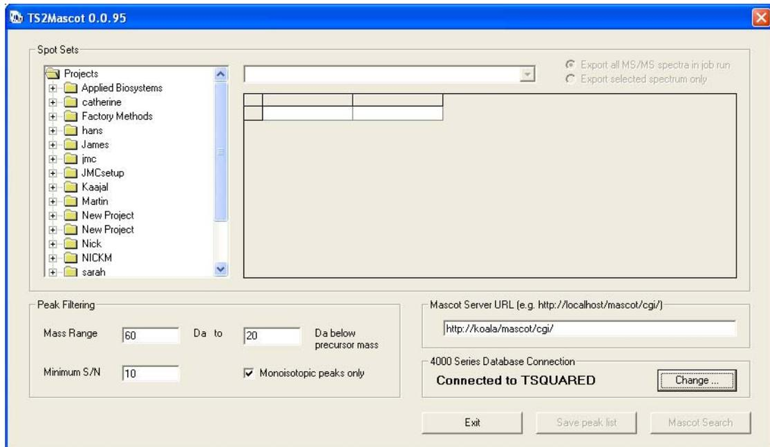
The Oracle service name is displayed towards the lower right. The folder tree in the *Spot Sets* frame is populated with project folders from the 4000 series database.
