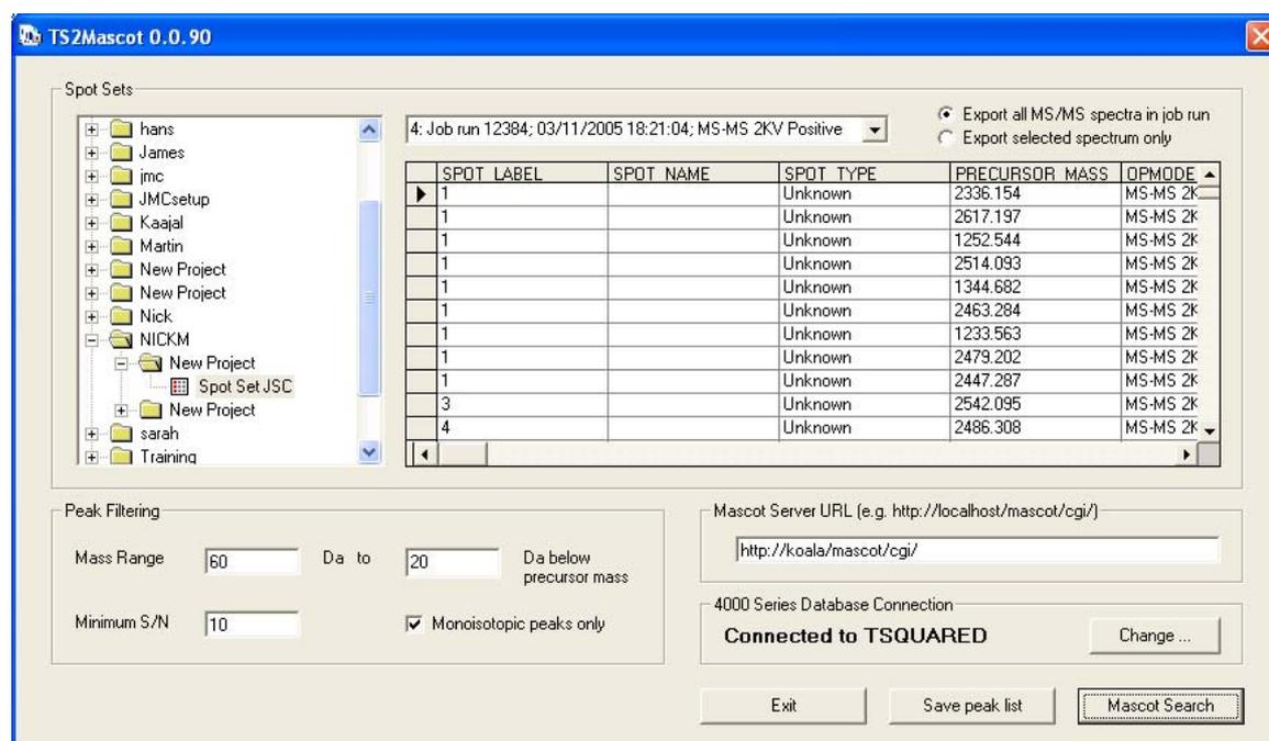
The radio buttons are used to choose whether to export all of the spectra in the job run, which only works for MS/MS data, or a selected spectrum, which works for both MS and MS/MS. The selected spectrum is indicated by the marker in the first column of the grid. Click in this column to select a different spectrum.
